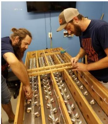
Other tasks included wiring over 500 brand new direct electric valve actions to a solid state computer. These replaced the older, damaged leather actions. All was tested properly before returning back to its Crown Heights home. Upon our return we removed the settled dust and gave the room a generous cleaning while releathering the wind reservoirs (bellows) that hold the air for the organ pipe chests.
